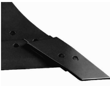
Points: The share points on Agrolux plough bodies are extra long and designed in such a way that wear is equal throughout the lifetime. The design means good soil contact, and new points will break through an eventual ploughing pan. The long point has exceptional wearing life with homogeneous dimension, The point, the share and the
